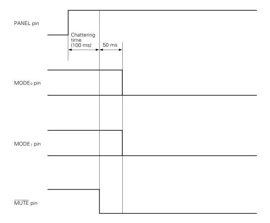
The mute output timing when the detachable panel is turned ON is the same as when the CE pin is turned ON.
